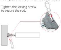
WALL FIXING: The fixing bracket is provided already assembled and ready for installation. Simply attach it to the wall with 2 D5 screws and corresponding plugs. We recommend mounting the shelves on a suitable support (particleboard, bricks, concrete, wood, ...).
